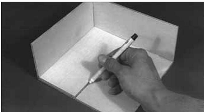
□ 8. Glue one side in place, lining it up with the edge of the bottom and the side of the back. Lay another side in the drawer as shown in the photo and mark along the edge. Remove the side and apply glue to two adjacent edges. Glue the side in place along the line you just drew.
