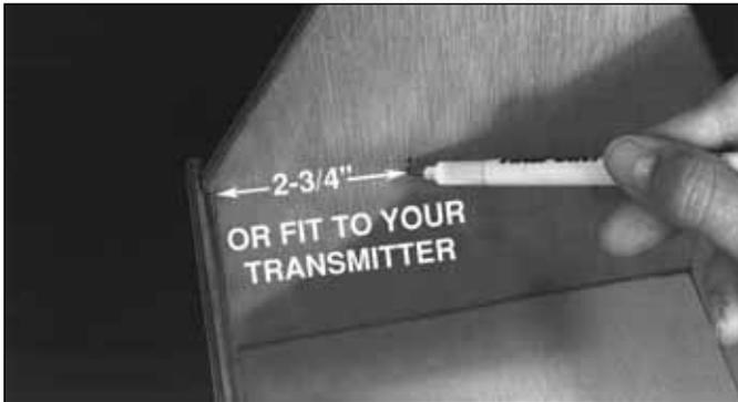
□ 12. Make a mark on both insides of the uprights, 2-3/4" from the side opposite the drawer. This is where the shelf divider will be installed. Test fit the divider in place and use your transmitter to make sure it is spaced correctly. When satisfied with the positioning, glue it in place.
