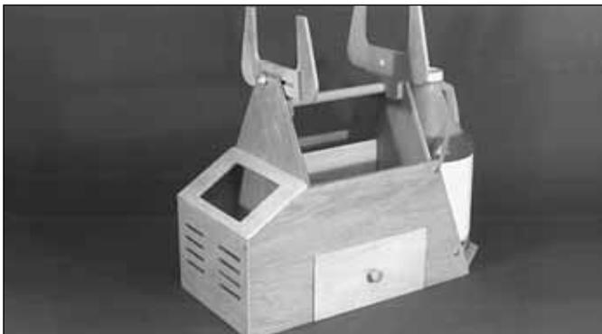
□ 24. Test fit your 12 volt battery in place and glue some leftover pieces of wood around it to keep it from sliding around and to help keep the battery upright. A couple of extra pieces of foam cradle cushion can be glued to the inside of the vented battery cover to help keep the battery upright.
