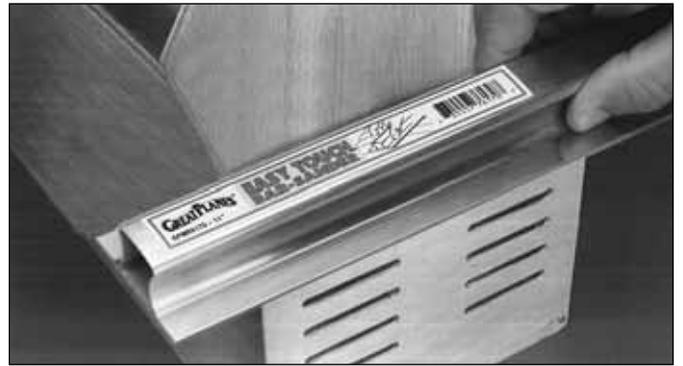
□ 15. Use a **flat** sanding block or the Great Planes® Easy-Touch™ bar sander to sand the sides and top edge of the panel flush with the sides of the box.
